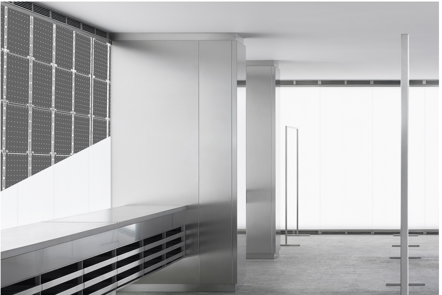
WOMEN'S WEAR DISPLAY AREA: a 20ft (6m) wall with vertical runs of 7 full TILES plus one cut-to-fit TILE at bottom of each run. The remote mounted drivers were located in the basement for accessibility.
